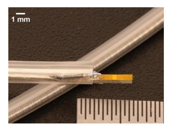
Researchers from North Carolina State University and the University of North Carolina at Chapel Hill have developed an ultrasound device to help identify arterial plaque that is at high risk of breaking off and causing heart attack or stroke. Credit: Xiaoning Jiang, North Carolina State University
