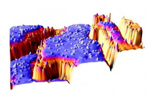
This shows tiny step edges on tungsten oxide surfaces. Credit: TU Wien
