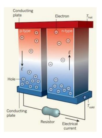
Working principle of a thermoelectric generator. Credit: (c) Nature, VOL 508, 327
