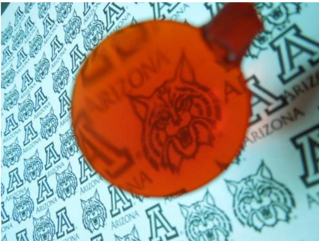
A University of Arizona-led research team has discovered a simple process for making a new lightweight plastic from the inexpensive and abundant element sulfur. This plastic can be molded into easy-to-make, lightweight lenses that transmit infra-red light. Credit: Jared Griebel/ Pyun lab, University of Arizona department of chemistry and biochemistry.
