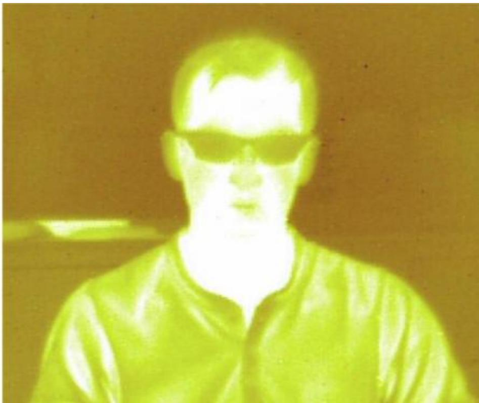
A thermal image of University of Arizona researcher Jared Griebel taken through a piece of new sulfur-based plastic using an infrared camera. Courtesy of Eustace L. Dereniak, University of Arizona College of Optical Sciences. Credit: Courtesy of Eustace L. Dereniak, University of Arizona College of
