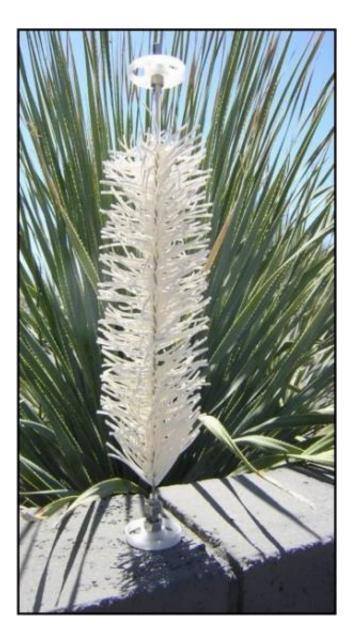
The artificial tree is able to absorb carbon dioxide when dry, and release it when moist.
