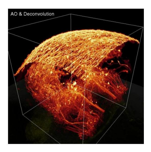
This image is a frame grab from a video showing imaging from an adaptive optics (AO) microscope operating in two-photon excitation (TPE) mode.
