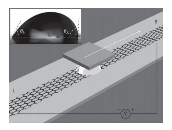
Illustration of the experimental set-up. A liquid droplet is sandwiched between graphene and a SiO2/Si wafer, and drawn by the wafer at specific velocities. Inset: a droplet of 0.6 M NaCl solution on a graphene surface with advancing and receding contact angles of 91.98 and 60.28, respectively. Credit: *Nature Nanotechnology* (2014) doi:10.1038/nnano.2014.56
