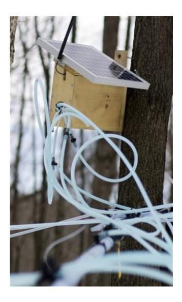
In this photo taken Friday March 21, 2014, one of maple syrup producer Donnie Richards wireless radio unit box containing sensors that monitor pressure on sap lines is seen in Milton, Vt. Richards has about 5,000 taps, with about 18 miles of tubing spread out over more than 100 acres and uses the wireless sensors to monitor the flow of sap that provides information immediately on a smart phone of tablet computer. (AP Photo/Holly Ramer)
