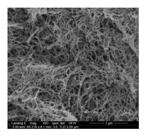
An electron microscope image shows the tangle of fibers contained in a hydrogel created at Rice University that could help clotting and heal wounds after surgeries. The Rice lab of bioengineer Jeffrey Hartgerink invented the synthetic peptides that self-assemble into fibers. Credit: Hartgerink Group/Rice University
