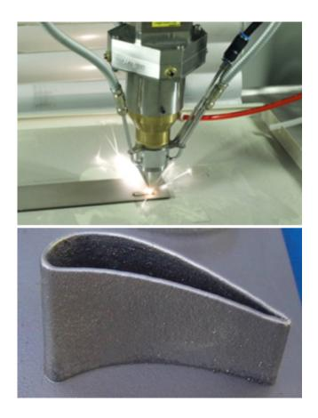
Laser-aided additive manufacturing (LAAM) (top) can be used to create complex structures such as airfoils (bottom) — used in the development of aircraft wings — from high-strength alloys. Credit: A\*STAR Singapore Institute of Manufacturing Technology
