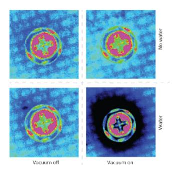
Dmitry Isakov at A\*STAR is investigating the infiltration of water under the surface of an aircraft by applying a vacuum to a bolt head. Thermal imaging reveals a cooler area around the bolt head when the vacuum is switched on (bottom right) that indicates the presence of water, which is not seen in a dry bolt head (top right). Credit: A\*STAR Singapore Institute of Manufacturing Technology
