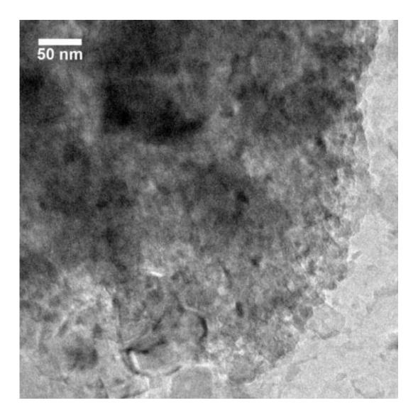
This is a micrograph of mesoporous silicon with sodium chloride and potassium chloride salts embedded in the matrix. Credit: Donghai Wang, Penn State
