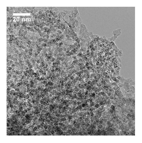
This is a micrograph of mesoporous silicon showing holes where salts were removed. Credit: Donghai Wang, Penn State
