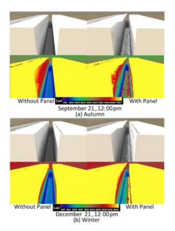
This is a simulation of the illuminance of an alleyway at noon at two different times of year, autumn (top) and winter (bottom). The new light-directing panel increases the amount of light that reaches the alleyway, as indicated by the higher amounts of red and yellow in the right-hand images ('with panel') compared to the left-hand images ('without panel'). Credit: *Optics Express*.
