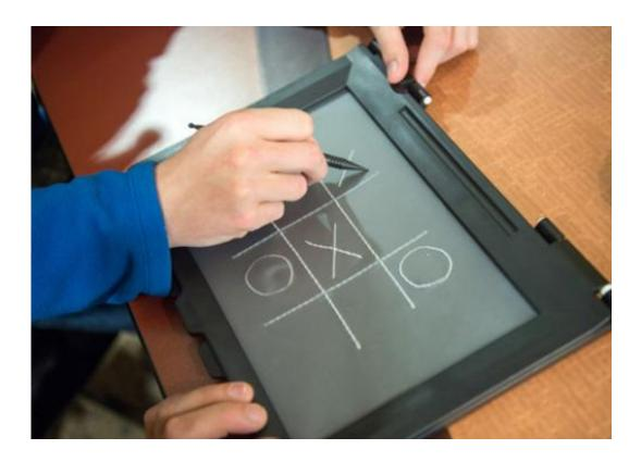
The inTACT Sketchpad allows blind and visually impaired users — for the very first time — to change, correct and update tactile graphics as they sketch. Credit:
