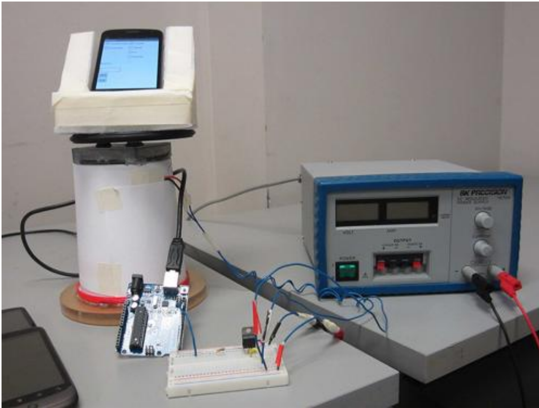
Experimental setup showing the external motor used for smartphone rotation. Credit: University of Illinois at Urbana-Champaign
