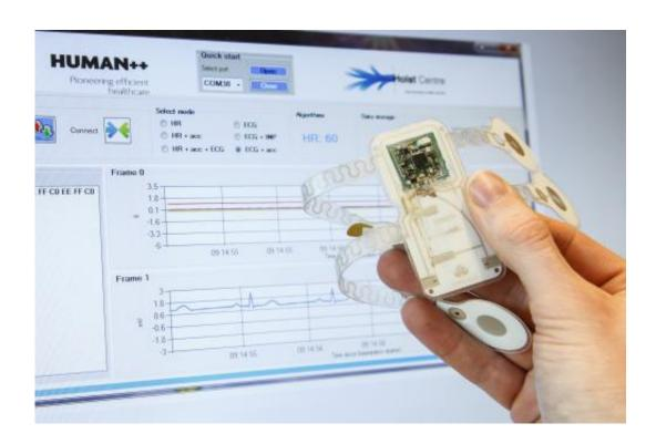
Holst Centre and IMEC have unveiled a prototype flexible health patch weighing just 10g – half the weight of current products. The patch uses real-time electrocardiogram (ECG), tissue-contact impedance and accelerometer information to accurately monitor physical activity. Thanks to advanced system in package (SiP) technology from ShinkoElectric Industries, the electronics module measures less than two
