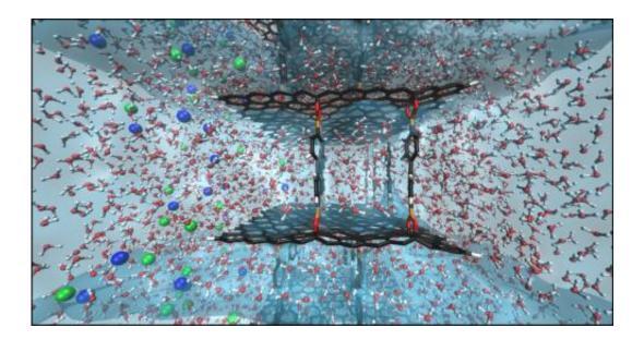
Simulations by Oak Ridge National Laboratory and Rensselaer Polytechnic Institute reveal the potential of graphene oxide frameworks, pictured in black, to remove contaminants such as salt ions, seen in blue and green, from water. Credit: Adrien Nicolaï/RPI.
