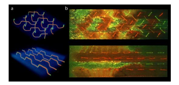
(a) X-ray computed micro-tomographic image reconstructions of "herringbone" (top) and "parallel" (bottom) vascular networks; (b) Fluorescent images of resin (red) and hardener (green) healing agent distributions across a delamination surface showing increased mixing (orange-yellow) effectiveness of the interpenetrating herringbone design. Credit: Jason Patrick
