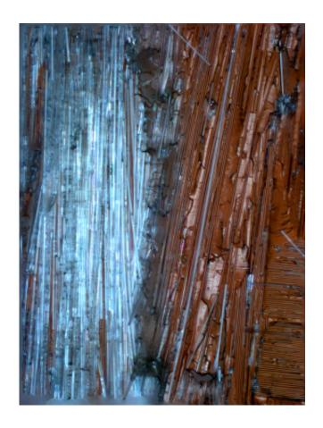
This is an optical microscope image of healed fracture surface showing landscape of ruptured glass fibers (left) and a portion covered with polymerized healing agents (right). Credit: Jason Patrick
