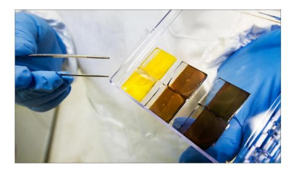
The band gap of perovskites can be adjusted by changing their compositions to access different parts of the sun's spectrum. Credit: Dennis Schroeder
