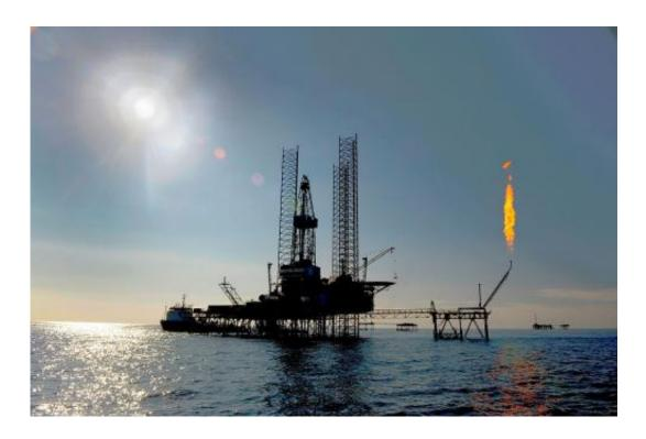
A jack-up drilling rig has tubular legs that support the deck and hull, and when positioned over the drilling site, rest on the sea floor. Credit: Wikimedia Commons
