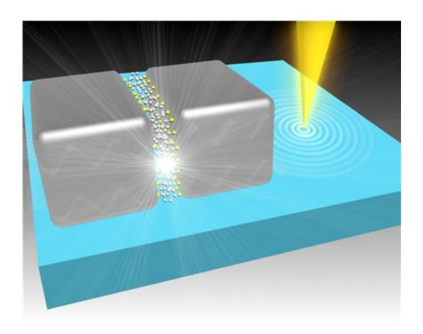
A focused electron beam (in yellow) was used to characterise the structures and to probe the optical properties of two plasmonic resonators bridged by a layer of molecules with a length of 0.5 nm. Credit: Tan Shu Fen, National University of Singapore
