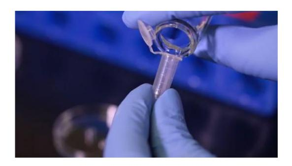
A McMaster team has reduced the sophisticated chemistry required for testing water safety to a simple pill, by adapting technology found in a dissolving breath strip. Want to know if a well is contaminated? Drop a pill in a vial of water and shake vigorously. If the colour changes, there's the answer.
