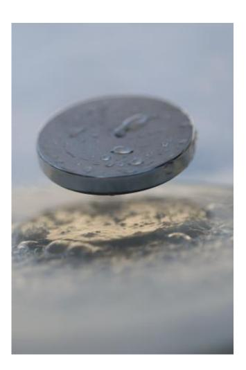
Superconducting materials expel magnetic fields, whose repulsive force can levitate a magnet, as shown here. Nevertheless, studies have shown superconductivity and magnetism can coexist in the same material. Now SLAC and Stanford researchers show that the two phases are interwoven at a very fine, microscopic level in a type of high-temperature superconductor known as an iron pnictide, and reveal how one phase gives way to the other. Credit: Julien
