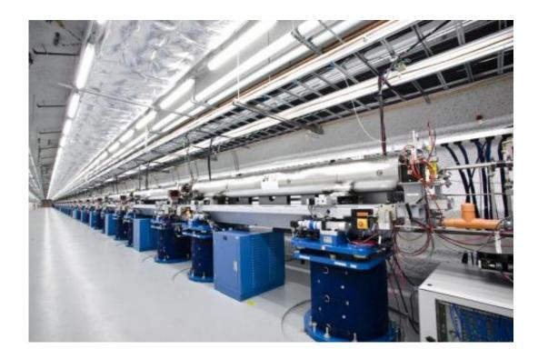
The Undulator Hall of SLAC Lab's Linac Coherent Light Source, which "wiggles" electrons to generate the high-power coherent x-rays crucial to this study.
