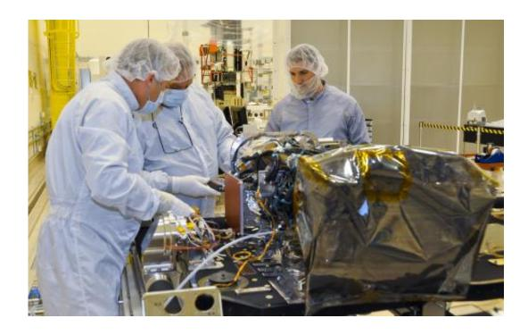
Lockheed Martin engineers in Denver install the Solar Ultraviolet Imager (SUVI) on the GOES-R Sun Pointing Platform. SUVI was built at the Lockheed Martin Advanced Technology Center in Palo Alto, Calif.
