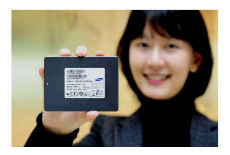
Utilizing Samsung's 10 nanometer (nm)-class\* 3-bit NAND flash components and advanced controller technology, the new drive features a sequential read speed of 530 megabytes per second (MB/s), while writing sequentially at 420MB/s. It also will read data randomly at 90,000 IOPS and handle sustained random writes at 14,000 IOPS.
