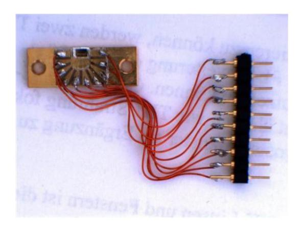
Laser chip mounted on a heat sink. The chip with several terahertz quantum-cascade lasers is soldered in the middle of a U-shaped contact pad with attached electrical leads. Credit: PDI
