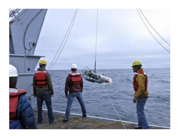
Oceanographers lowered their instrument into the canyon in April 2013. The tool was built to measure fast-moving water close to the seafloor. Credit: Parker MacCready, UW
