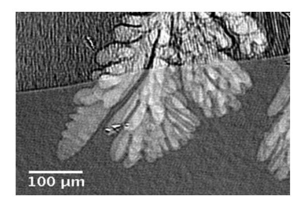
An x-ray image of a 200 micron thick aluminum-14 atomic percent copper alloy during directional solidification, highlighting the growth of an aluminum-rich branched structure (dendrite) and the advancing solid-liquid (planar) interface. The advancing lamellar eutectic solid consists of two different phases.
