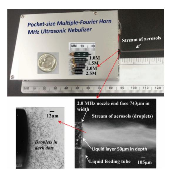
This is a pocket-size ultrasonic nebulizer with insets: (Top) Nebulizer and MEMS-fabricated MHz nozzles laid on its cover. (Bottom) Aerosols ejected from the medicinal liquid layer resting on the end face of the nozzle tip: (L) Individual aerosols imaged using a high-speed camera (104 frame/sec) with short
