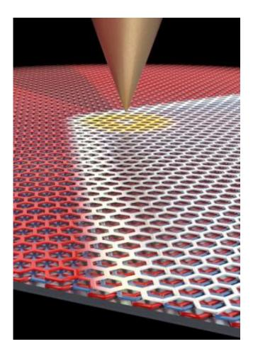
Using a sharp metal scanning tunneling microscopy tip, LeRoy and his collaborators were able to move the domain border between the two graphene configurations around. Credit: Pablo San-Jose ICMM-CSI
