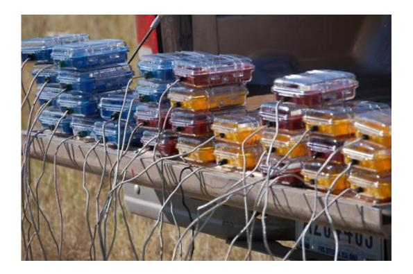
Thermocouples (the silver wires) and data loggers are used in prescribed burns in research plots planted with purple threeawn. The loggers record plant temperatures every second the fire burns. Credit: Mark Jacobsen, Bureau of Land Management.
