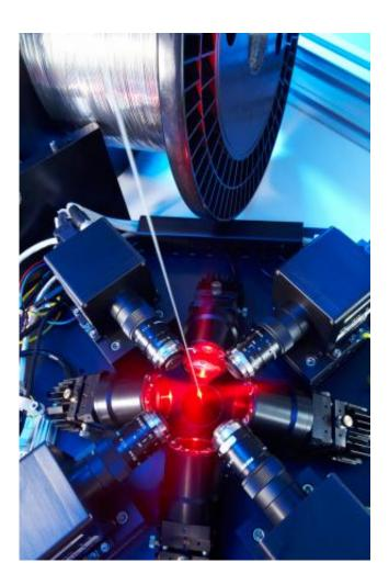
With the WIRE-AOI wire inspection system, four cameras collectively deliver 40,000 analyzed images per second. Thus, a 100% control of the wire surface in real time can also work with very rapid production processes. Credit: Fraunhofer IPM
