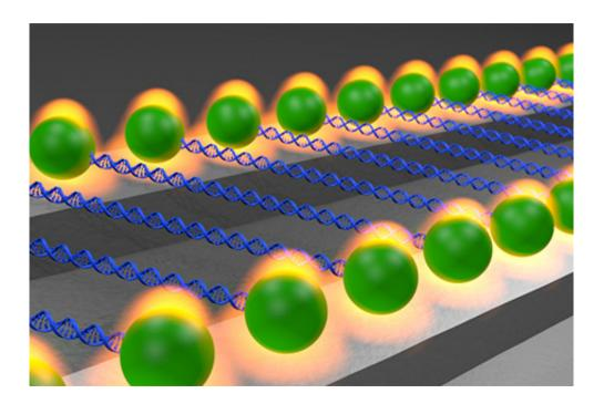
An illustration of a nanophotonic standing wave array trap (nSWAT) for parallel manipulation and measurements of single molecules. Here, an array of DNA molecules with a bead attached at each end is precisely manipulated between two nSWATs. The position of each nSWAT is independently controlled to relocate and transport the array of trapped beads. Credit: Robert Forties
