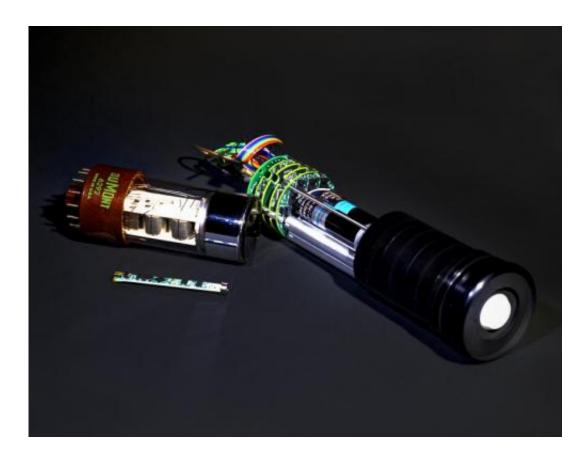
The fully assembled OCULLAR prototype is pictured on the right. A legacy photomultiplier tube is shown on the top left. A new silicon photodetector microradiometer is on the bottom left. Credit: NASA Goddard/Bill Hrybyk
