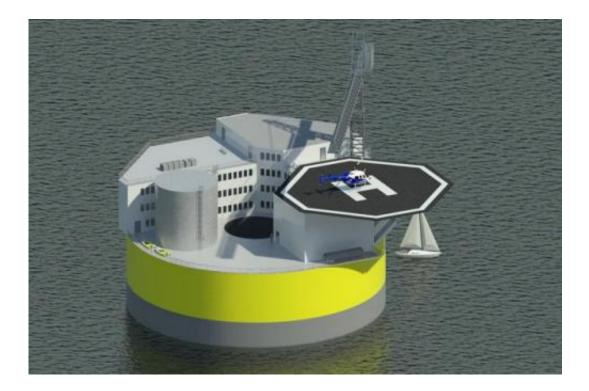
This illustration shows a possible configuration of a floating offshore nuclear plant, based on design work by Jacopo Buongiorno and others at MIT's Department of Nuclear Science and Engineering. Like offshore oil drilling platforms, the structure would include living quarters and a helipad for transportation to the site. Credit: Jake Jurewicz/MIT-NSE
