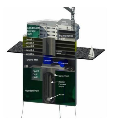
Cutaway view of the proposed plant shows that the reactor vessel itself is located deep underwater, with its containment vessel surrounded by a compartment flooded with seawater, allowing for passive cooling even in the event of an accident. Credit: Jake Jurewicz/MIT-NSE
