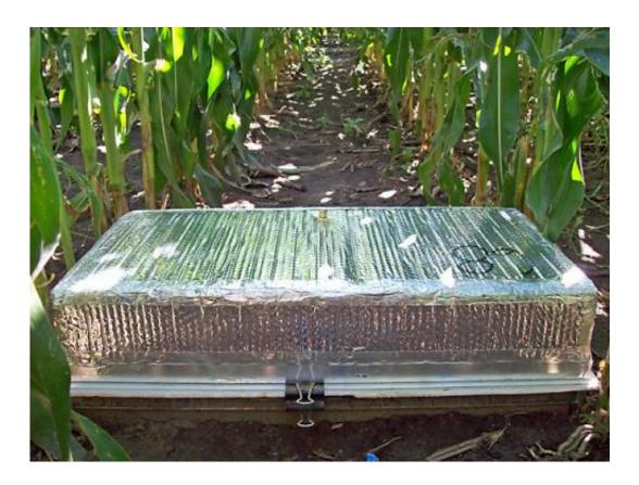
A covered gas flux chamber from a study done in a field of maize during two growing seasons. The study examined the effects of different nitrogen fertilizer sources and application methods on nitrous oxide emissions. Credit: Rodney Venterea
