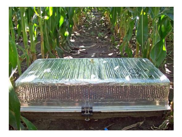
A covered gas flux chamber from a study done in a field of maize during two growing seasons. The study examined the effects of different nitrogen fertilizer sources and application methods on nitrous oxide emissions. Credit: Rodney Venterea
