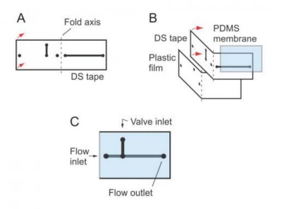
Double-sided tape is cut with channels and ports that will align when folded (A). The polymer membrane that supplies the valve function for the microfluidic device is sandwiched between (B). The completed apparatus (C) has ports for fluid flow into and out of the device, as well as a valve inlet for air. Air pressure pushes the membrane into the flow channel, blocking fluid movement. Credit: Gregory A. Cooksey/National Institute of Standards and Technology
