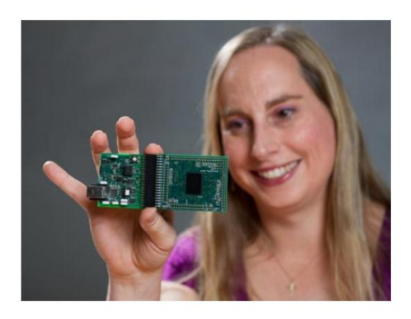
Professor Jennifer Hasler displays a field programmable analog array (FPAA) board that includes an integrated circuit with biological-based neuron structures for power-efficient calculation. Hasler's research indicates that this type of board, which is programmable but has low power requirements, could play an important role in advancing neuromorphic computing. Credit: Rob Felt
