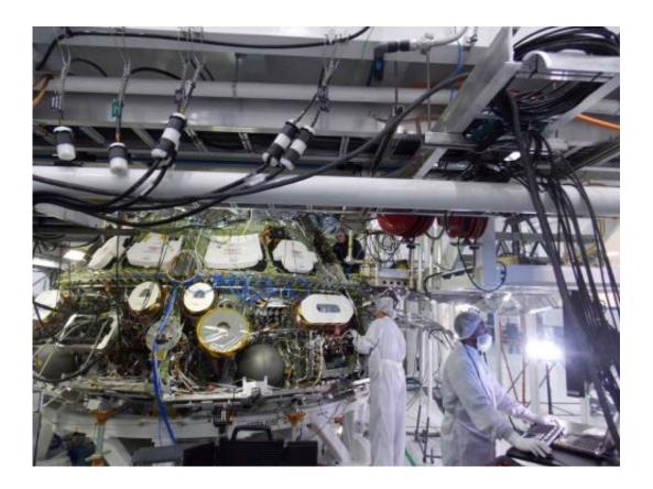
Engineers in the Operations and Checkout Building at NASA's Kennedy Space Center in Florida, perform avionics testing on the Orion spacecraft being prepared for its first trip to space later this year. Credit: Lockheed Martin
