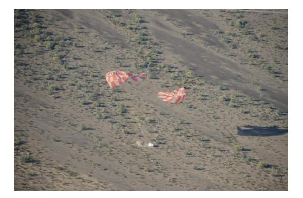
Orion's parachutes deflate after a successful touchdown following a test at the U.S. Army's Yuma Proving Ground on April 23. Credit: NASA
