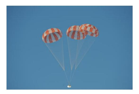
A test version of Orion descends under its three massive main parachutes, which together would cover almost all of a football field. Credit: NASA
