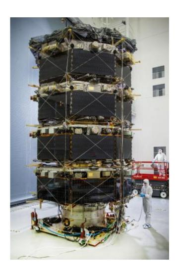
All four stacked Magnetospheric Multiscale, or MMS, spacecraft with solar arrays are ready to move to the vibration chamber at NASA's Goddard Space Flight Center in Greenbelt, Md., where they will undergo environmental tests. Credit: NASA/Chris Gunn
