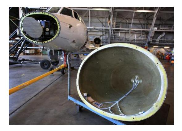
Equipment in the nose of the Guardian will precisely measure wind velocity when the jet flies through the wing tip wake vortices of a DC-8 during ACCESS-II flight tests. Credit: NASA Langley / David C. Bowman
