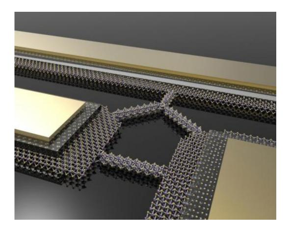
This is a molecular model showing the structure of the nanowires created out of a monolayer of transition-metal dichalcogenides (TMDCs). Credit: Junhao Lin, Vanderbilt University
