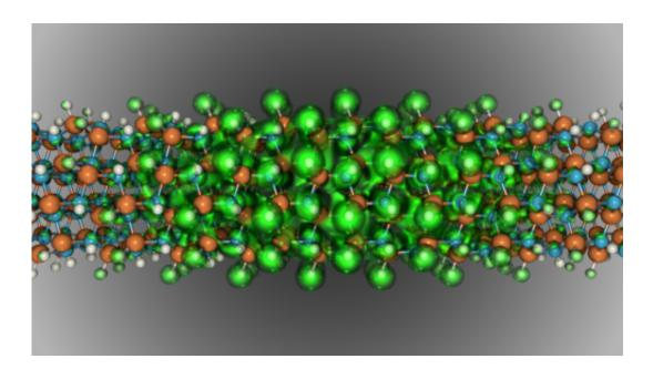
This simulation of a one-nanometer wide Indium Nitride wire shows the distribution of an electron around a positively charged 'hole.' Strong quantum confinement in these small nanostructures enables efficient light emission at visible wavelengths. Credit: Visualization: Burlen Loring, Lawrence Berkeley National Laboratory
