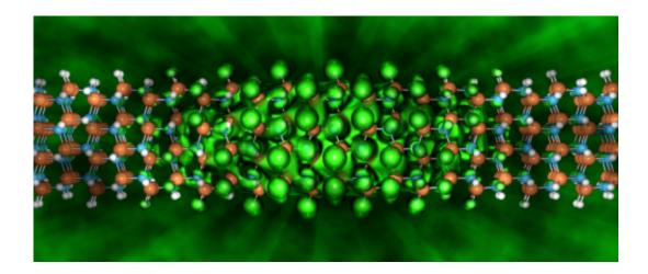
(Alternate view) This simulation of a one-nanometer wide Indium Nitride wire shows the distribution of an electron around a positively charged 'hole.' Strong quantum confinement in these small nanostructures enables efficient light emission at visible wavelengths. Credit: Burlen Loring, Lawrence Berkeley National Laboratory
