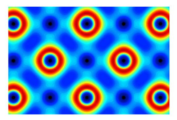
This image shows the resonant bonding in lead telluride, one of the materials whose properties the team studied. It shows the calculated electron density distribution within the material. Credit: Sangyeop Lee
