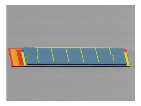
The top cell in the stacked 3-junction/germanium assembly captures wavelengths between 300 nm and 1,300 nm; wavelengths from 1,300 nm to 1,700 nm pass through to the bottom cell. Credit: Xing Sheng, University of Illinois
