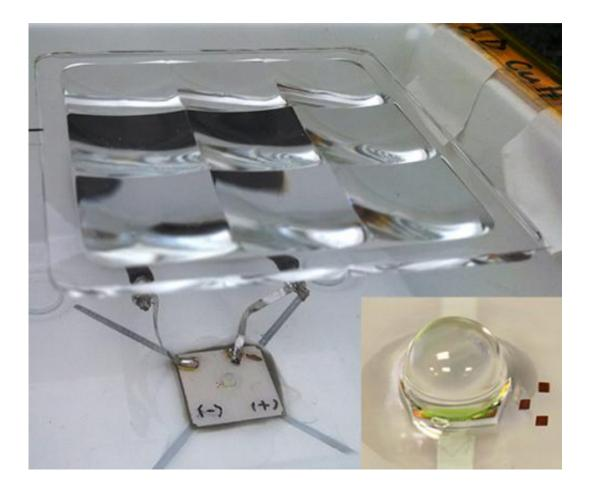
Dual-stage optics, consisting of a molded 2 X 2 cm2 primary lens and a secondary, 2 mm ball lens (inset) focus incident sunlight by more than one thousand times. Credit: Xing Sheng, University of Illinois
