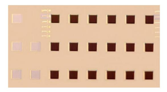
This shows printing-based assembly process yields arrays of stacked multijunction cells in a fully automated step-and-repeat mode with high yields and accurate overlay registration. Credit: Xing Sheng, University of Illinois
