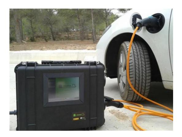
The Instituto Tecnológico de la Energía (ITE) in Spain has developed the first mobile charging system for electric vehicles. This system allows users to charge their vehicle from any plug -not just from a specifically designed one- as long as it has been previously authorised by an electric power company.
