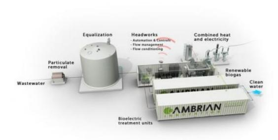
Layout of Cambrian Innovation's EcoVolt wastewater treatment system, which can generate enough electricity to meet 25 to 50 percent of a brewery's needs and produce about 25 percent of clean, reusable water. Credit: Cambrian Innovation
