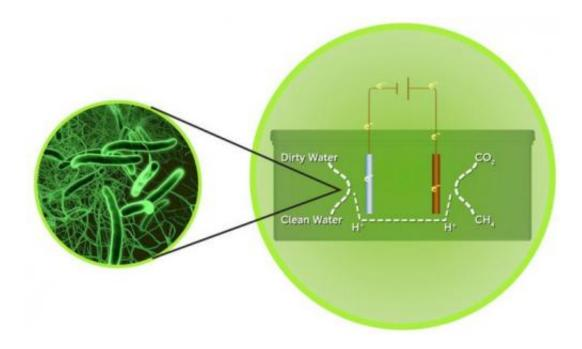
Inside the treatment units, exoelectrogens (at left) consume pollutants in the wastewater and create electricity. The electricity travels through a circuit for other microbes to consume — along with carbon — to produce burnable methane. Credit: Cambrian Innovation
