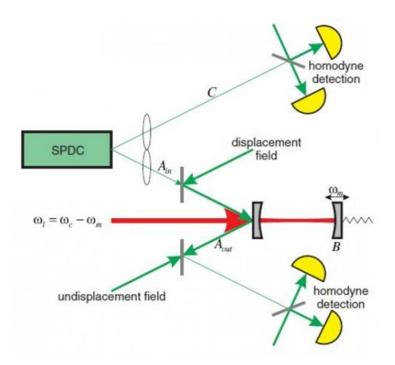
Proposed setup for generating optomechanical "cat states," a form of micromacro entanglement in which the quantum states of photons and phonons are in superposition. Credit: R. Ghobadi, et al. ©2014 American Physical Society
