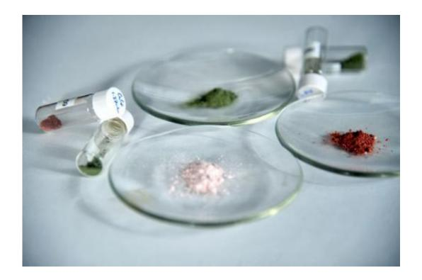
The porphyrin-functionalized organosilicate sorbents Dr. Brandy White desgined at NRL capture and break TIC/TIM and other targets down into things that are harmless. "Air purification technology could be in the ductwork of the building, it could be on stack gases for exhaust from industrial processes," she says. Credit: U.S. Naval Research Laboratory/Jamie Hartman
